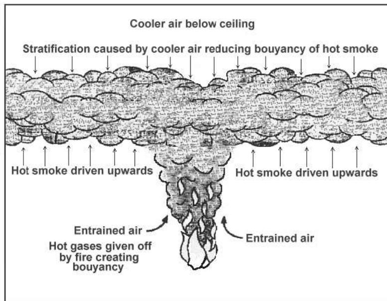
The upward movement of smoke in the plume is dependent upon the smoke being buoyant relative to the surroundings. The potential for stratification relates to the difference in temperature at the ceiling and floor levels of the open space. There is a maximum height to which plume fluid (smoke) will rise, especially early after ignition, depending on the convective heat-release rate and the ambient temperature variation in the open space.
